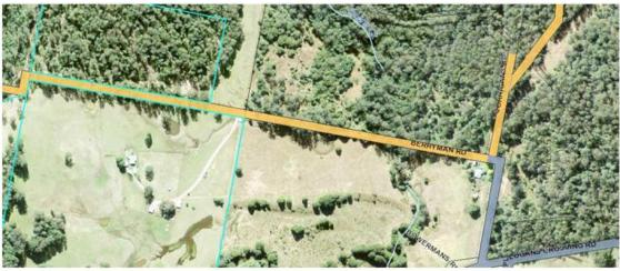
Logans Crossing Road is a sealed road of two-lane width without kerb and gutter, which is owned and maintained by Council. Council's records indicate that Logans Crossing Road has a 'Rural Local Major' AUS-SPEC classification. The proposal will result in an increase of one equivalent tenement (ET) as a result of the subdivision, or less than 7 vehicle trips per day on average, which is within the capacity of this road.
