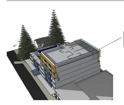
EXTENT OF ROOF THAT EXCEEDS THE HEIGHT LIMIT AND IS ADDRESSED IN THE DA REPORT, asking PMHC to permit the in crease in roof height under the provisions of Clause 4.6
