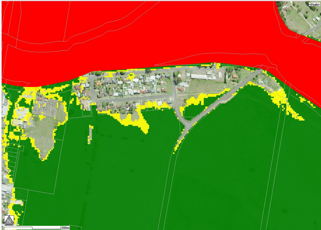
2016 Flood Study Scenario 1 Flood Hydraulic Categories (Note: there is no change to the Floodway extent).
