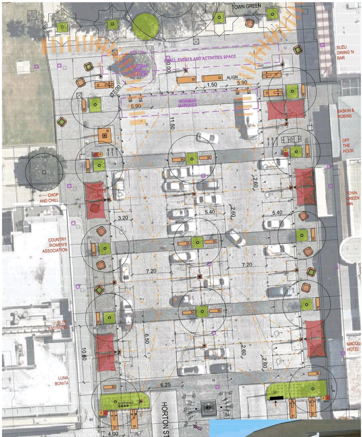
PLAN 1. MAKMAX PERMANENT UMBRELLA CANTILEVER DOUBLE SHARED POST SQUARE 4X4M (14.5m 2 ) ON EXISTING LIGHT POLE FOOTING ? T.B.C.
