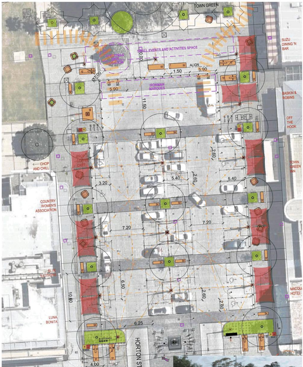
PLAN 3. CENTER POLE SQUARE 4X4M (16m 2 ) PERMANENT - 1100x1100x400 FOOTING FOLD DOWN - 800x800x150 FOOTING IN PAVEMENT BASE COURSE
