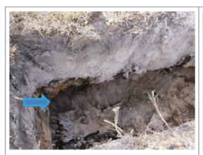
TP2 – Typical profile with aeolian sands, overlying a thin upper indurated sand horizon, overlying more aeolian sands. The test pit is collapsing due to water inflow occurring above a lower indurated sand layer (not visible).
