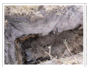
TP2 – Typical profile with aeolian sands, overlying a thin upper indurated sand horizon, overlying more aeolian sands where the test pit is collapsing due to water inflow occurring above a lower indurated sand layer.
