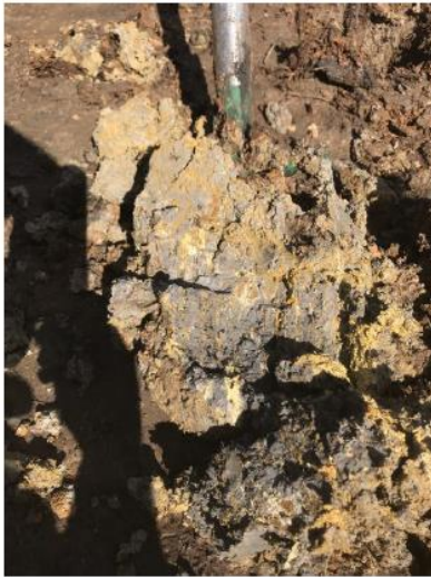
Photo 2: Yellow mottling indicating the presence of jarosite in actual acid sulfate soils clays. Site LI-6.
