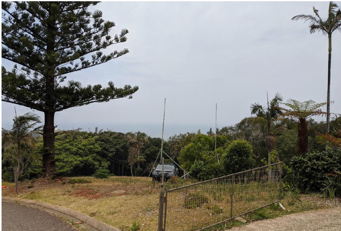
Figure 3: Height poles in the location of the two proposed height exceedances. The pole to the right of frame has a total height of 9m (0.5m or 5.8% exceedance), whilst the pole to the left has a total height of 8.76m (0.26m or 3% exceedance).
