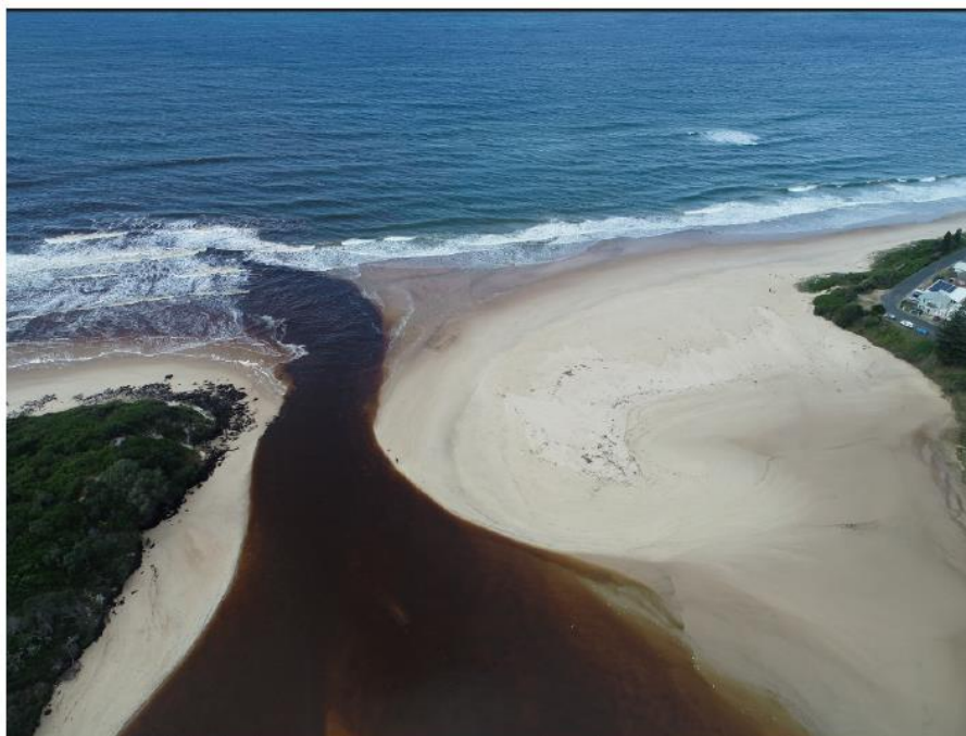
Figure 4: The Lake Cathie entrance opening showing a width of approximately 35m to 40m on the 29 May 2020.
