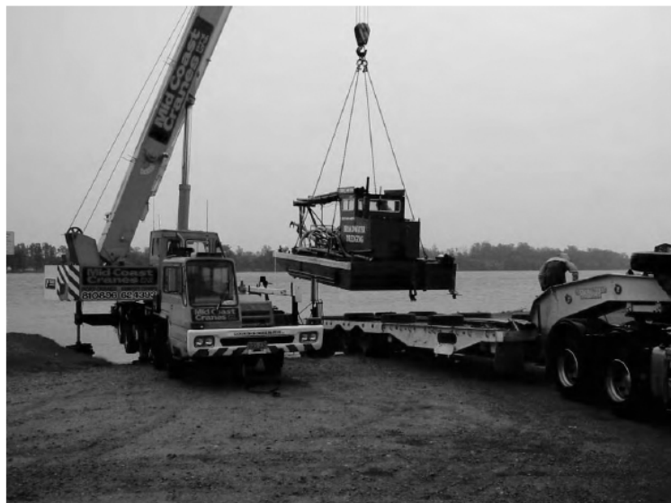
Figure 2: Small truck-mounted CSD used in 2006 maintenance dredging campaign
