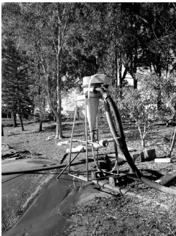
Figure 3: Hydrocyclone unit used in 2006 maintenance dredging campaign
