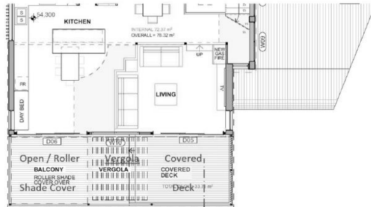
Figure 15: Plan View of the variety of roof coverings proposed for the existing deck
