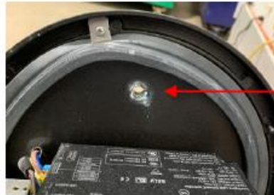
Water pooling in frame outside sealed area
