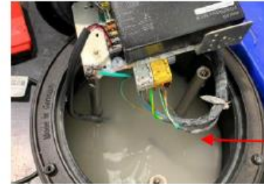
Corrosion on frame as a result of water pooling
