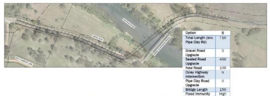
Figure 15 - Option B: New Bridge immediately upstream of existing bridge
