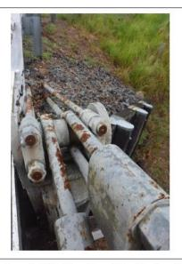
Photograph 104 - Overview of Steel Anchor Rods
