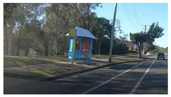
Figure 6.1: Indented Bus Stop with Shelter
