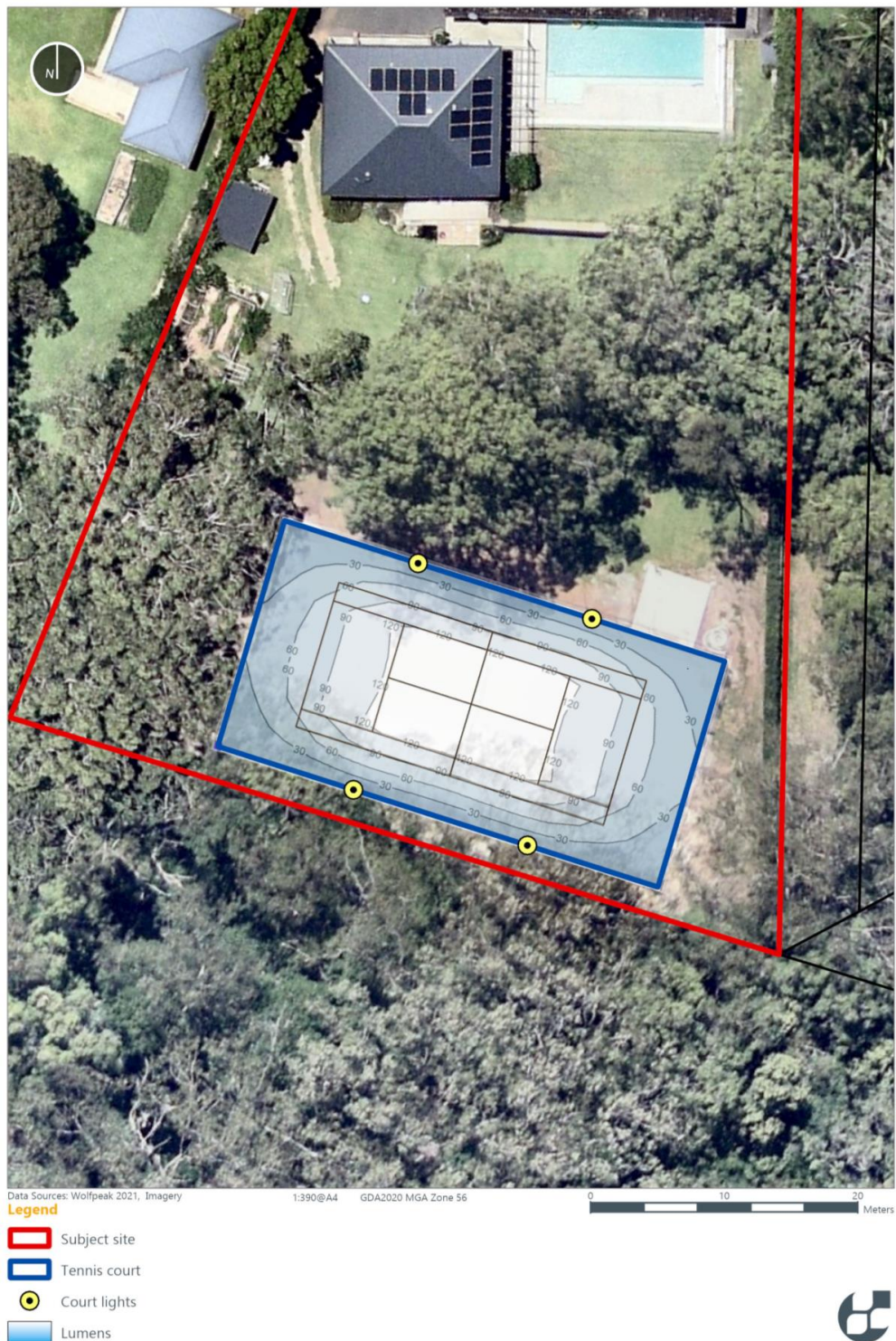
Figure 4: Extent of lumens from proposed lighting within tennis court fencing
